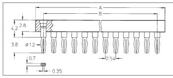
546-91-xxx-xx-xxx-035 546-93-xxx-xx-xxx-035 546-99-xxx-xx-xxx-035 PGA sockets with press-fit terminations for 2.1 to 3.2 mm PCB thickness. Hole diameter 1 (+0.09/-0.06) mm
